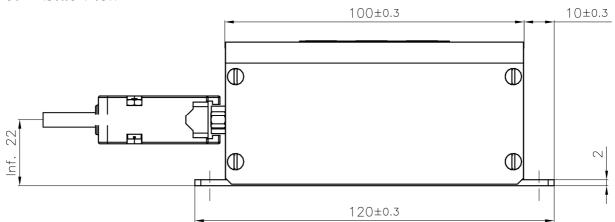
NOTE: All measurements are in millimeters. The view shows the Flight Recorder with plugged connector.
