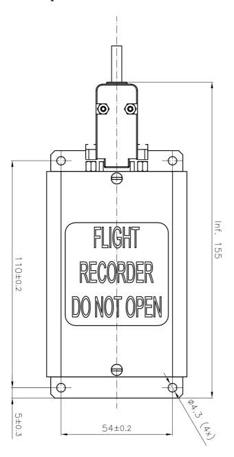
NOTE: All measurements are in millimeters. The view shows the Flight Recorder with plugged connector.
