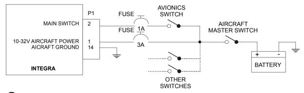
Protection by fuse of pin no.2 is recommended as it is shown on picture. The reason is protection against accidental short circuit caused by connector manipulation or failure of cable insulation.
