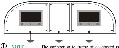
**NOTE:** The connection to frame of dashboard is recommended, because the metal case of Integra is in contact with metal plate of dashboard. In case dashboard is not connected to frame and onboard systems are simultaneously connected to dashboard, current would flow through the case of Integra and it may result in damage of the Integra.
