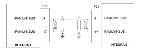
**CAUTION:** A twisted pair cable must be used to connect instruments or equipment within the iFamily® CAN BUS system.
