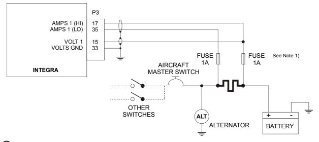
**(i) NOTE 1:** Protection by fuse is recommended as it is shown on picture. The reason is protection against accidental short circuit caused by connector manipulation or failure of cable insulation.
