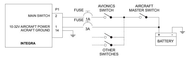
**(i) NOTE:** Protection by fuse of pin no.2 is recommended as it is shown on picture. The reason is protection against accidental short circuit caused by connector manipulation or failure of cable insulation.
